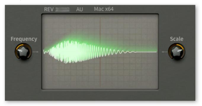
The scope displays a mono sum of the output, before the Delay effect. The *Frequency* knob on the left adjusts horizontal resolution, while the *Scale* knob on the right adjusts vertical resolution.
