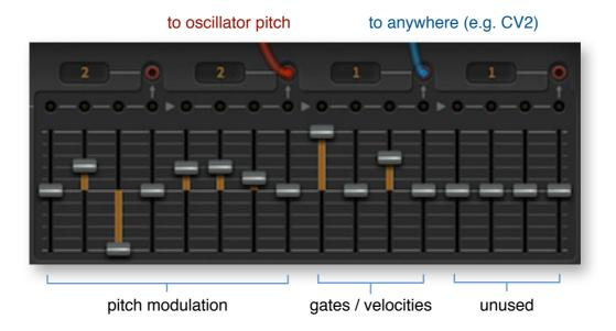
The first 8 values control oscillator pitch via the red cable, while the blue cable is connected to CV2 (for instance). Even if the signal is not used, this second tap **must be connected** to something (anything), otherwise *ModSeq2* would remain undefined.
