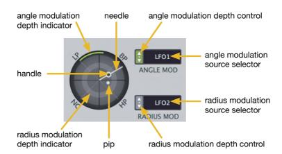
The **needle** position (a.k.a. angle) specifies the mixture between two of the four filter modes: In the above image it is mostly BP plus a little HP... at least it would be if the small **handle** along its length were at the rim! With the handle positioned fairly close to the centre, a significant amount of the 'opposite' filter modes (NC and LP) is blended in. Note: you don't have to grab the handle to move the needle.
