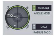
negative radius modulation depth is indicated by a darker ring that moves towards the centre
