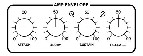
**Volume Curve** trimmer: In the original hardware, the VOLUME knob controls how much amp envelope modulates the final VCA. It also affects the envelope **curvature** – not by design, but as a side-effect of how it works. As Repro-1's equivalent **OUTPUT** knob comes after all effects, the only way to implement this quirk was as a separate control – the trimmer between DECAY and SUSTAIN.
